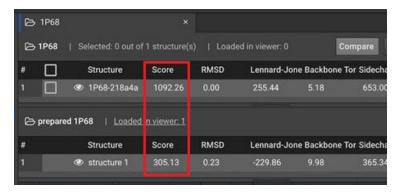
The comparison above shows that after the Prepare function was run the Score for the energy of the 1P68 structure was lowered from a score of 1092.26 to 305.13 Rosetta Energy Units
